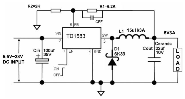
Fig10. TD1583 Typical Application Circuit (with ceramic output capacitor) @ 5V/3A
