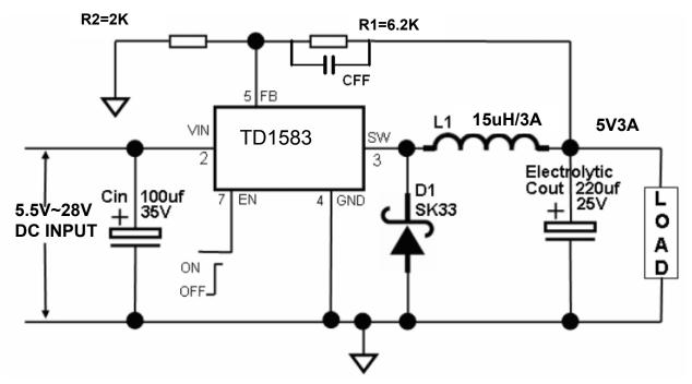
Fig8. TD1583 Typical Application Circuit @ 5V/3A
