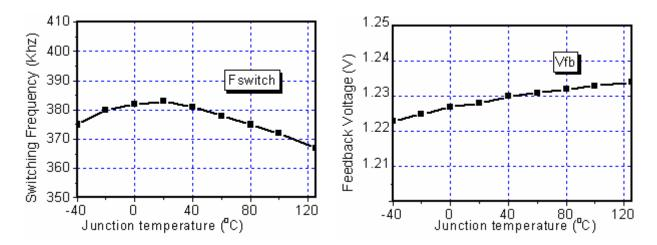
Figure 4. Switching Frequency vs. Temperature
