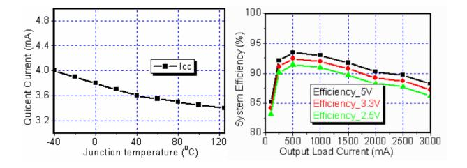
Figure 6. Icc vs. Temperature
