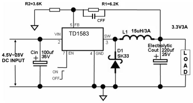
Fig9. TD1583 Typical Application Circuit @ 3.3V/3A
