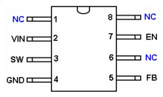
Figure 2 Pin Configuration of TD1583 (Top View)
