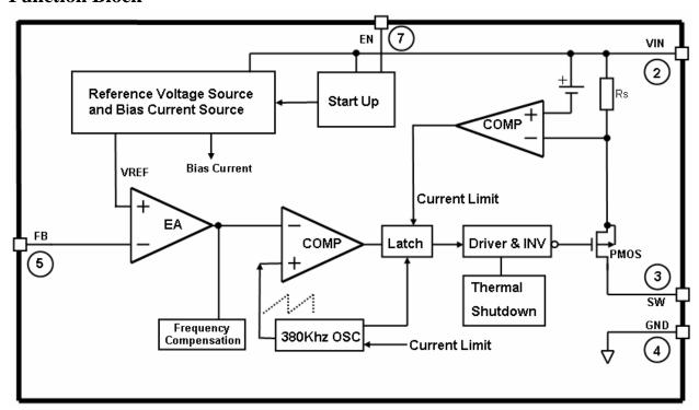
Figure 3 Function Block Diagram of TD1583
